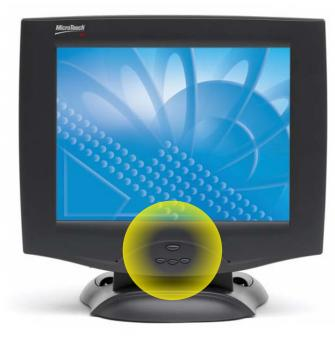
Locking OSD controls avoid accidental or unauthorized display adjustments
