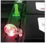
Exclusive rotating 2-color LED "snail" clips show charging status and can also serve as hold down clips for battery, if needed.
