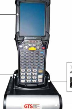
**Dual-chemistry charger** Supports Li-Ion and Li-Polymer chemistries.
