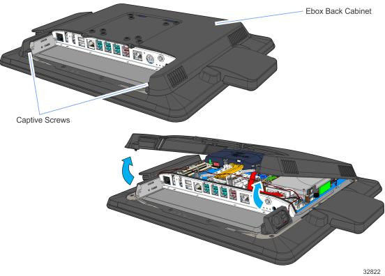
2. The optional Hard Disk Drive is mounted on the inside of the Rear Cover. If an HDD is present, disconnect the HDD Power and Data cables from the motherboard.
