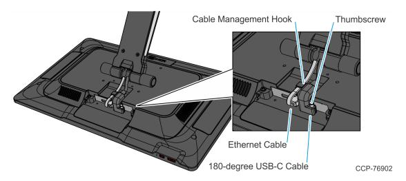
4. Remove the two (2) captive screws that secure the Back Cover to the Display.
