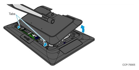
6. Install the Memory Module in the Memory Socket at an angle as shown.
