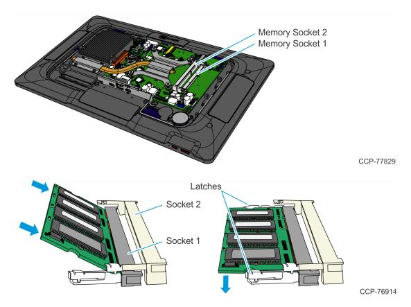
7. Press the Memory Module down until it latches in position. Ensure the latches are completely engaged.
