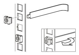
*To remove:* Remove any attached screw and reverse the action in step 2. Grasp the caged nut before releasing the tool.
