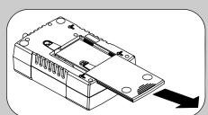
Slide the battery compartment cover completely onto the Back-UPS ES.
