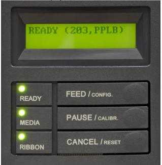
The multi-function operation panel and LCD screen makes installation, configuration, and operation simple and convenient. The LCD screen can also display information in Spanish, French, German, Italian, Portuguese, or Simplified Chinese.
