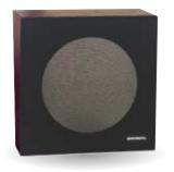
Bogen's wall baffle is ruggedly constructed of 3/8" particle board with reinforced corners. It is finished in simulated walnut and will house any of our 8" speakers. A sloping front panel provides enhanced downward dispersion. Hardware for mounting a speaker to the baffle included.
