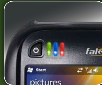
Status LEDs: power, scan and keyboard status
