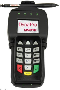
Secure cryptographic device for PIN, with SCRA, EMV contact / contactless, and optional contactless NFC, signature capture, and privacy shield
