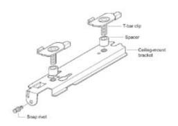
Figure 1: Ceiling Mount Bracket Kit
