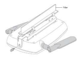
Figure 2: Mounting Access Point to T-Bar
