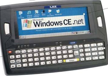
Large 6.5" (165mm) 1/2 VGA, LCD color display w/touch screen for crystal-clear viewing and easy data entry.
