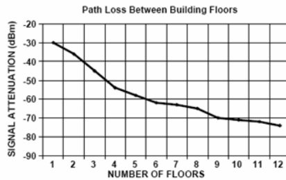
Figure 7. Attenuation Between Floors
