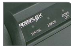
Three LED colour indicators for status display.
