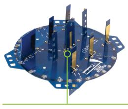
A patented smart antenna array integrates six high-gain vertically-polarized and six horizontally-polarized antenna elements. This enables up to 4096 potential antenna combinations and up to 9 dBi gain, thereby delivering unprecedented range extension and signal reliability. The dual polarized smart antenna increases the effectiveness of spatial-multiplexing, resulting in higher data rates.
