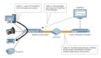
Figure 1. Flexible secure wired access deployments
