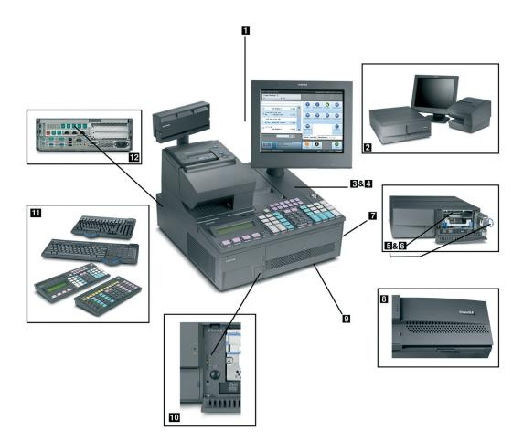
1 Shown: SurePOS 785 with 12 in. SurePoint display, SureMark dualstation printer, 67-key Keyboard with LCD, and 40-character display
