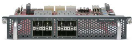
7008XLS Media Dependent Adapter featuring 8 x 10GBASE-SFP+ sockets
