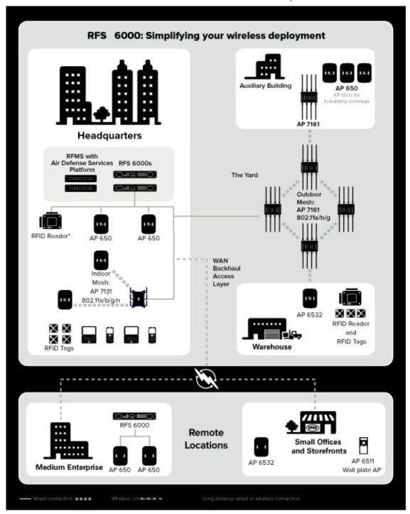
The RFS 6000 offers the comprehensive functionality necessary to extend wireless voice, video and data access inside medium to large enterprises — as well as to remote locations such as branch offices.
